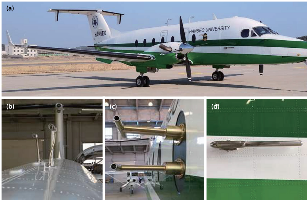
Fig. 1. Aircraft measurement platform: (a) Beechcraft B1900D, (b) aerosol inlet, (c) trace gas inlet, (d) meteorological sensor.
