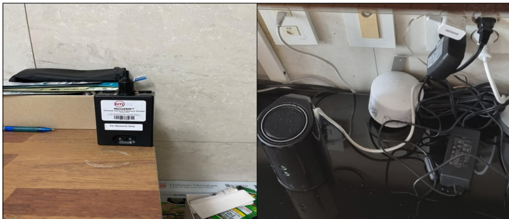
Fig. 1. MicroPEM (left) and PurpleAir (right) placed in a participant's living room during the indoor PM_{2.5} monitoring campaign conducted across 68 households in 2023.
