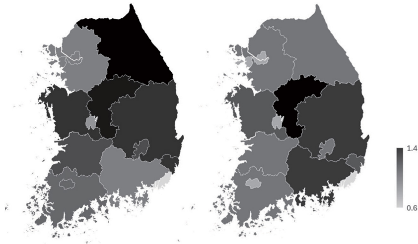
Fig. 2. Operating-to-registered VKT ratio (left: passenger, right: freight).
