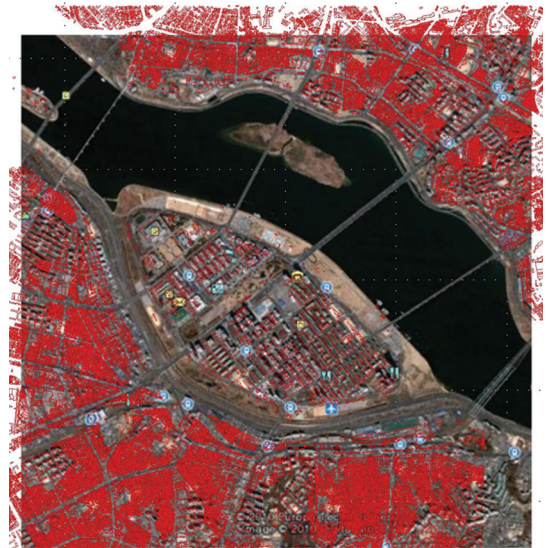
Fig. 1. The modeling domain of 5 km×5 km horizontal dimensions : 32,159 buildings, red polygons overlapped against the satellite image are located in the modeling domain.
