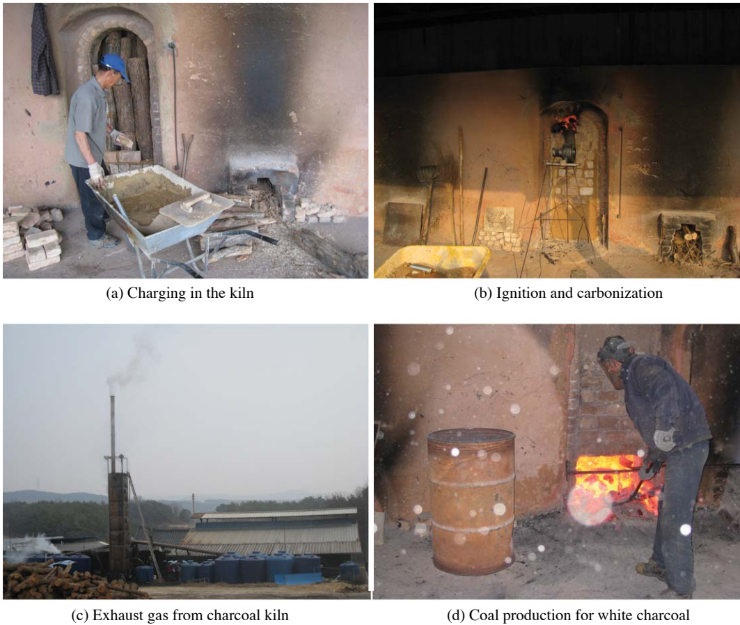
Fig. 2. Charcoal production in commercial scale kiln.
